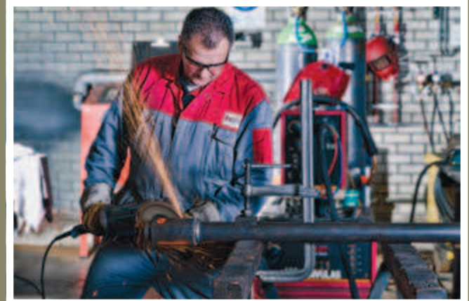
A sterntube's mounting aids are welded on in our workshop.
